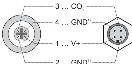
1) GND internally connected
